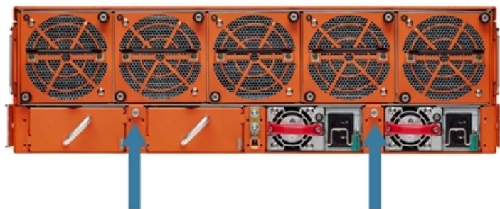
Figure 10 Fan Tray Screw Location on GigaVUE-HC3 Rear
