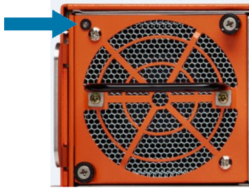
Figure 6 Individual Fan LED Location on GigaVUE-HC3 Rear
